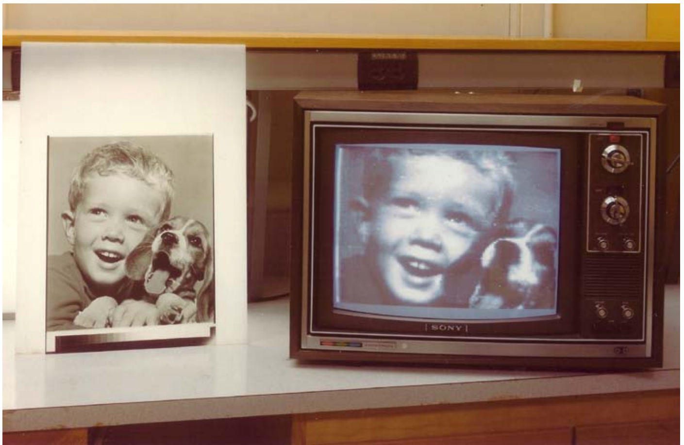
Figure 2 Steven J. Sasson, Setting of the test arrangement, in: Technical Report , 1977. © Eastman Kodak Company, Rochester.
